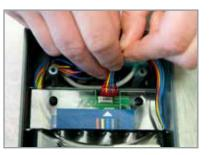
4. When you are sure that you have connected the lithium-ion battery in accordance with the instructions, screw the rear cover of the VAS 5581 back on. Your HV diagnosis box is now ready for use.
