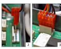
Attaching the plug in a manner contrary to the instructions specified above may cause defects, or result in a short-circuit, as soon as the VAS 5581 is switched on.
