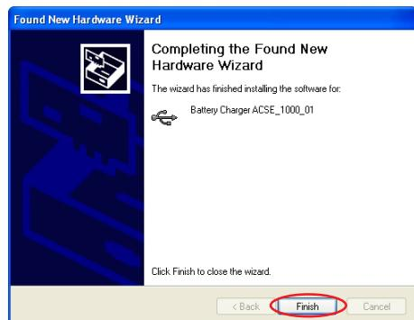
**Important:** For further devices, or when changing the USB connection, the device driver must be reinstalled.
