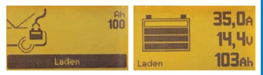
Charge batteries in the vehicle power circuit to a maximum of 14.4 volt and 35 ampere. Pre-selection of the battery rating and the model type (wet, AGM, gel). Permanent display of charge progress, mode of operation, and electrical values.
