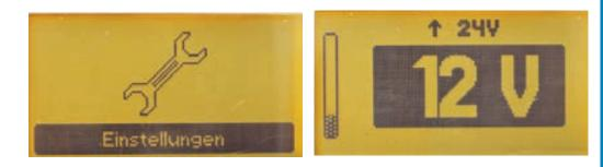
Easy user guidance thanks to the clearly arranged display and automatic detection of vehicle voltage.
